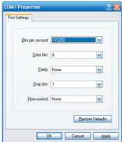
Figure 4-2 Tera Term COM Port Configuration
