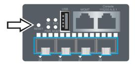
Figure 6-4: SGS-6341-16S8C4XR Reset Button
