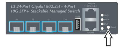
Figure 6-1: SGS-6341-24P4X Reset Button
