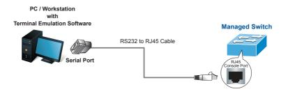
Figure 4-1 Managed Switch Console Connectivity
